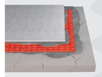
A ceramic tile system can be protected against the emergence of cracks by the simple inclusion of a disconnecting product. This ensures the continued durability of the ceramic tiles over time.
